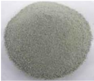
Figure 3-1. Photo of the Posiva MX-80 material Be-Wy--VTT002 (Kiviranta et al. 2011)
