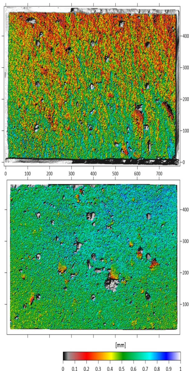
Figure 14 – Colored fracture aperture distribution at artificial granite block fracture (Jankovec J., 2019)
