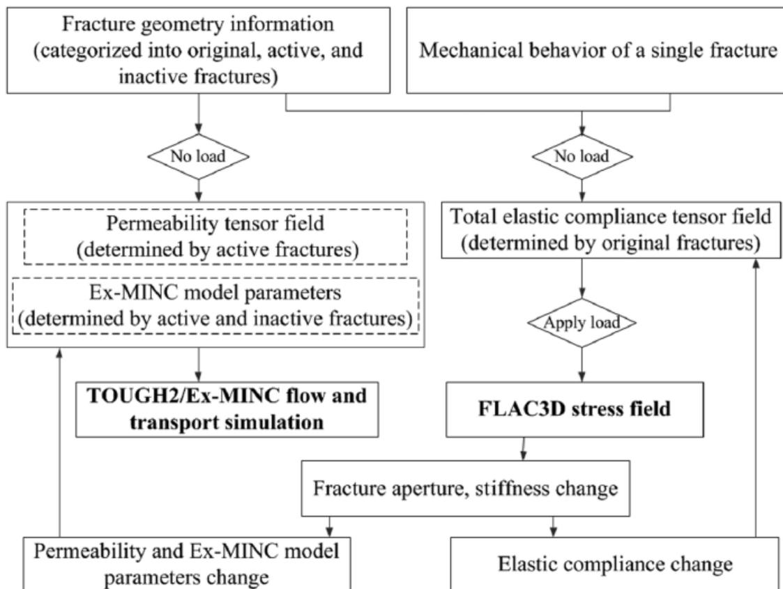
Figure 6: Scheme of the extended multiple interacting continua (Ex-MINC) method (Wang et al., 2014).
