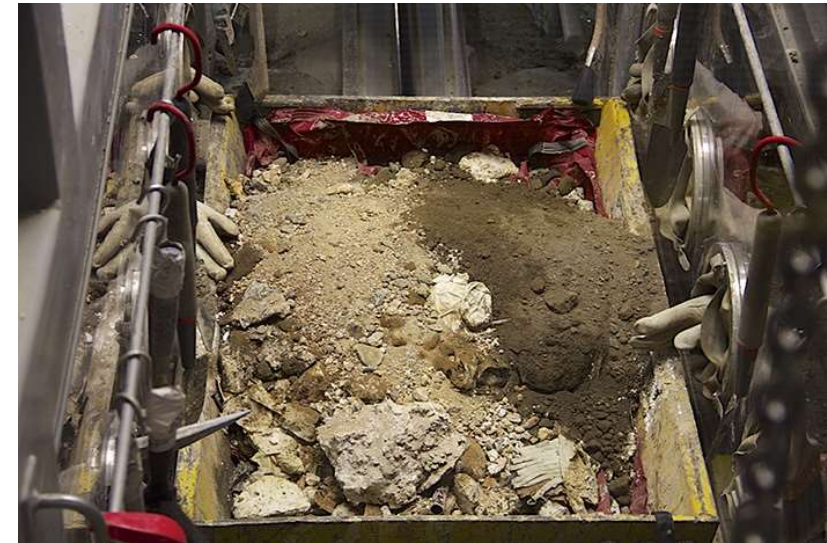
Targeted waste in a drum packaging station for visual examination, Idaho, USA., Source: USA DOE, 2016 article on Idaho clean-up, web page
