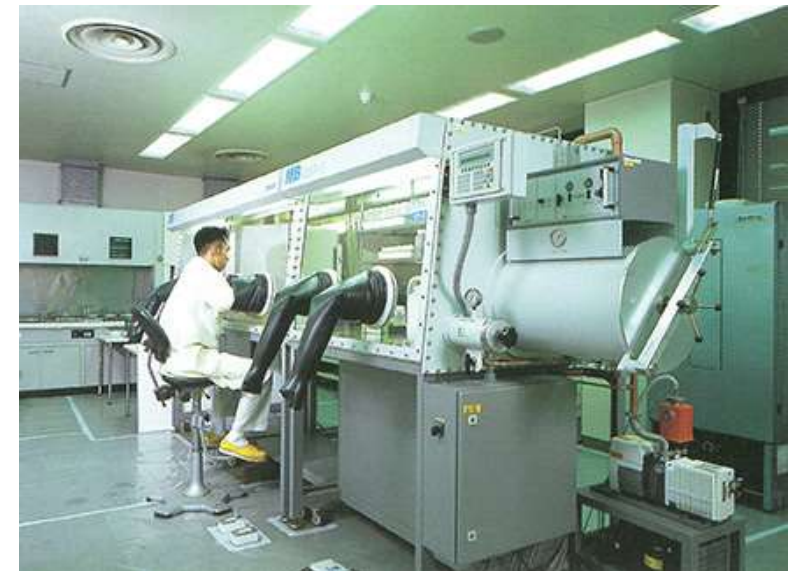
Inert gas glove box, used when characterizing materials, Source: JGC web
